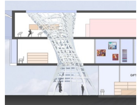
FIG. 7 Section showing the West core penetrating through the building for different public activity spaces.
